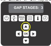
10. Using the "UP" key, select the desired AM/PM option and press the "ENTER" or "OK" key to accept.
