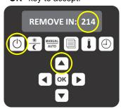
**12.** Using the "UP ARROW" key, select the "MANUAL" or "AUTO" options and press the "ENTER" or "OK" key to accept.
