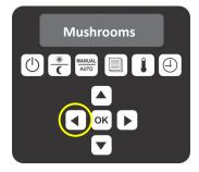
4. When in the "REMOVE IN" screen press the "TIME" key for 5 sec. The old menu item is removed and a new ADD ITEM will be added.
