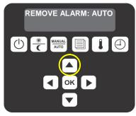
13. Using the same keys in Step 11, enter in your "REMOVE GAP" numbers. Press the "ENTER" or "OK" key to accept.
