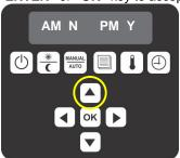
11. For the "REMOVE IN" option use the "ON/OFF" key to scroll left or right and the "UP ARROW" to change the number. Press the "ENTER" or "OK" key to accept.
