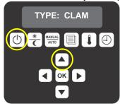
Using the "UP" key, select one of the gap stages options (0,1,2,3), and press the "ENTER" or "OK" key to accept.
