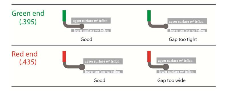
**Note:** This tool is for diagnostic purposes only and is not acceptable for performing gap calibration.
