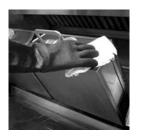
Rinse inner edges of platens. 20 Press the STANDBY button twice to lower the right platen. Rinse the inner edges of the right and left platens with a clean, sanitizer-soaked grill cloth. Press the RAISE button to raise the right platen. (Note: For 3 platen grills, lower the center platen.
