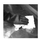
Apply oil to lower grill surface. 31 Apply a thin layer of fryer cooking oil to the lower grill
