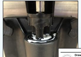
This is what happens when you don't clean and lubricate the spinner shaft seal properly during cleaning cycles and replace quarterly.
